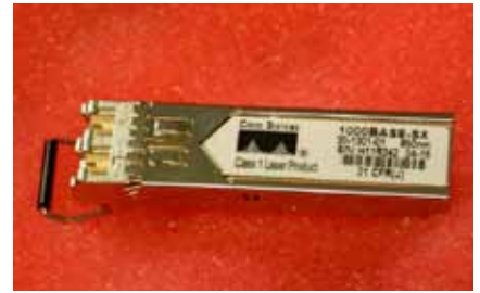
A confiscated counterfeit version of Cisco's Small Form-Factor Pluggable (SFP), a compact, hot-pluggable transceiver used for both telecommunication and data communications applications.
